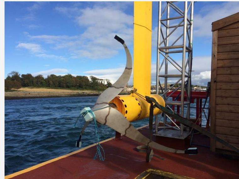
Figure 11 Tidal turbine manufactured by NSCC for Biome Renewables
